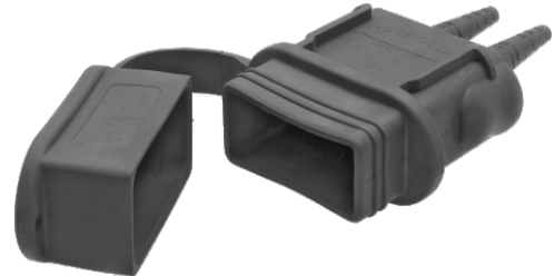
21125 Load end boot suit all 120A SC connectors. ● Rubber housing helps keep out contaminants to IP64 ● Mates with 21124 kit for an in-line sealed connection ● Tapered cable sleeves suits various diameter cables
