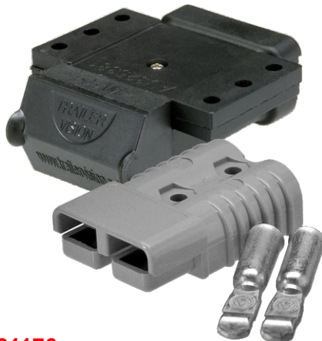
21176 Black 175A supply end surface mounting SC connector kit. ● Spring hinged lid and rear seal helps keep out contaminants ● Supplied with 21175 connector
