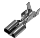
21500 Female locking terminal suit all male housings except 21511 & 215112 (use 56210) Quality tinned brass material. For cable up to 4mm auto.
