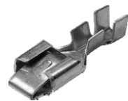
56209 Female locking terminal suit 21511 & 215112 housings. Quality tinned brass material. For cable up to 4mm auto.
