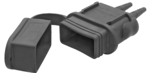
21181 Load end boot suit all 175A SC connectors. ● Rubber housing helps keep out contaminants to IP64 ● Mates with 21180 kit for an in-line sealed connection ● Tapered cable sleeves suits various diameter cables
