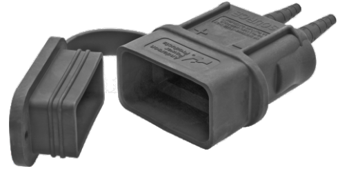
21124 Supply end boot suit all 120A SC connectors. ● Rubber housing helps keep out contaminants to IP64 ● Mates with 21125 kit for an in-line sealed connection ● Tapered cable sleeves suits various diameter cables
